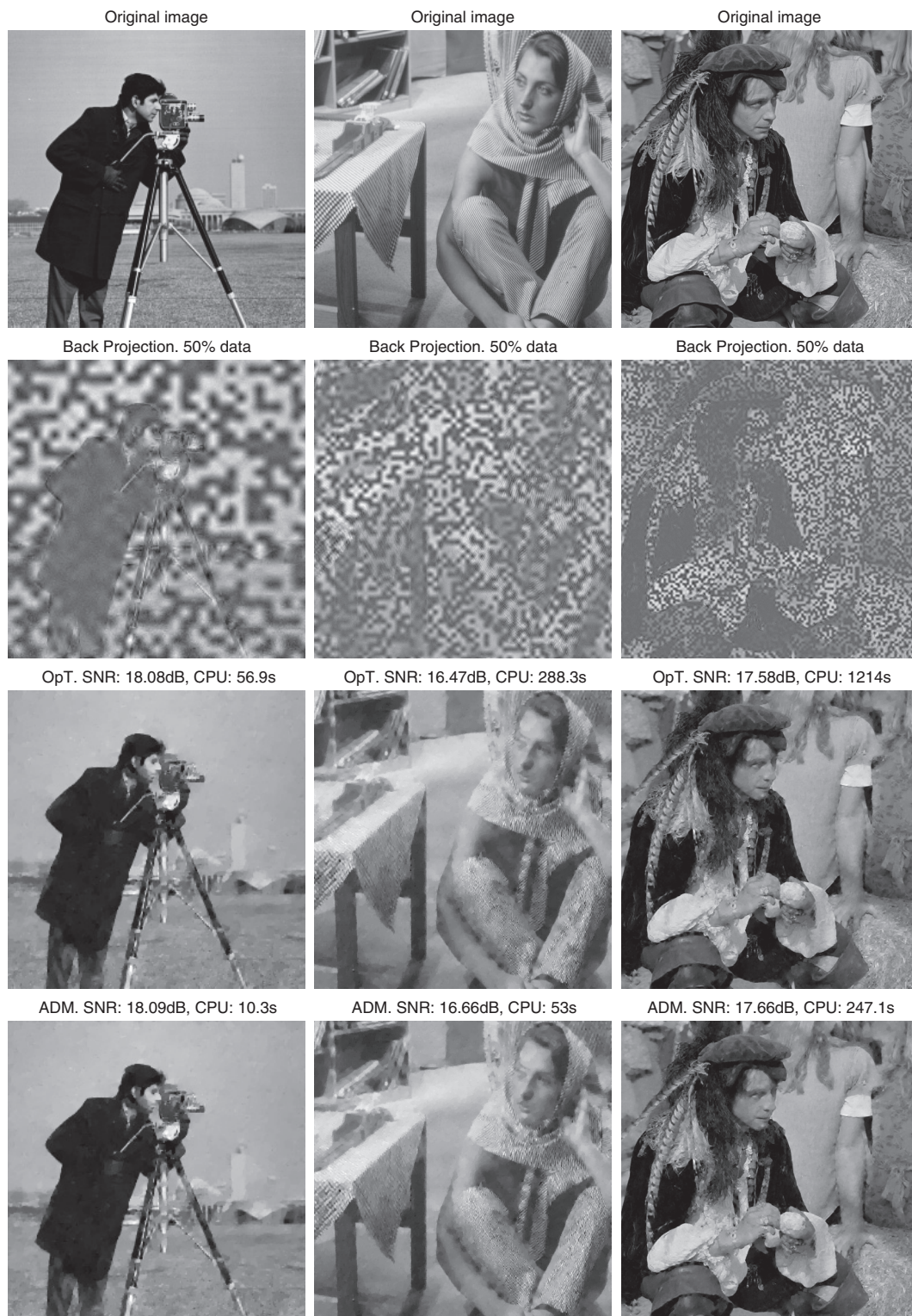
Figure 4. Images recovered by both algorithms from 50% wavelet coefficients. First row: original images. Second row: back projections. Third row: recovered by OpT. Bottom row: recovered by ADM.
