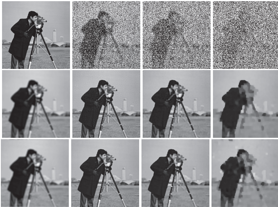
FIG. 4.1. First column from top to bottom: original Cameraman image, blurred image by Gaussian kernel of size 7 \times 7 and standard deviation 5 with the Neumann boundary conditions (SNR: 9.69dB), blurred image by the same kernel with periodic boundary conditions (SNR: 9.57dB), respectively; second to fourth column, top row: the blurry image is corrupted by 40%, 60%, and 80% salt-and-pepper noise, respectively; second to fourth column, middle row: results recovered by LAD method (CPU time: 491, 493, 905 seconds; SNRs: 14.47, 11.78, 8.08dB); second to fourth column, bottom row: results recovered by FTVd ( \epsilon \equiv 0.001 in (2.16); \mu = 36, 10, 2 ; CPU time: 31, 30, 32 seconds; SNRs: 14.81, 11.62, 8.09dB, respectively).
