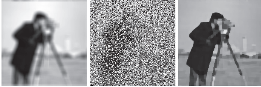
FIG. 4.2. Left: Cameraman image blurred by Gaussian kernel of size 15 \times 15 and standard deviation 9, SNR: 7.23dB; middle: the blurred image is corrupted by 60% salt-and-pepper noise; right: result recovered by FTVd ( \epsilon = 0.001 in (2.16); \mu = 10 , CPU time: 26 seconds, SNR: 10.38dB).
