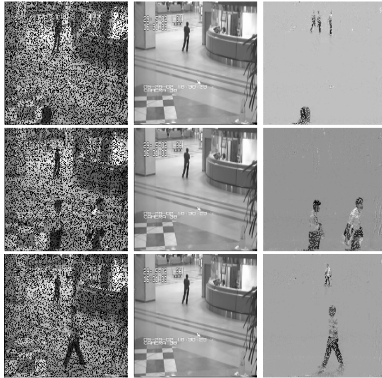
Figure 2: Background extraction from a noisy video with missing data
